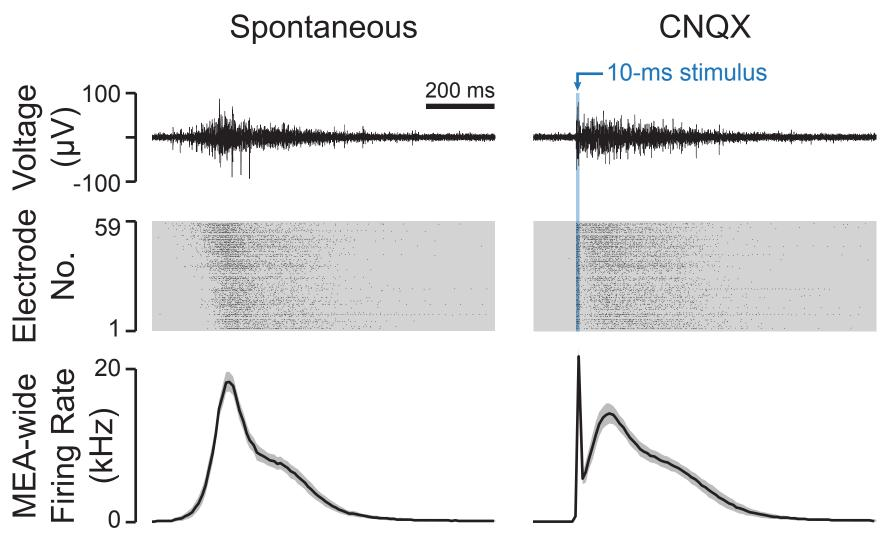
Figure 5: Bursts evoked during CNQX treatment resemble spontaneous bursts. Top, voltage recording on a single microelectrode during a spontaneous burst (left) or an optically-evoked burst during CNQX treatment (right). *Middle*, rastergram of spikes detected on all electrodes during bursts shown above. Bottom, average burst firing rate profile during 6-hour period before CNQX (left), or during 24-hour CNQX treatment with closed-loop optical stimulation (right). Shading, s.d.
